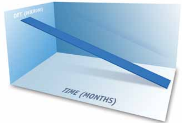
GRAPH 1: EXAMPLE OF POLISHING GRAPH – SIGMA SYLADVANCE 800 SYSTEM
