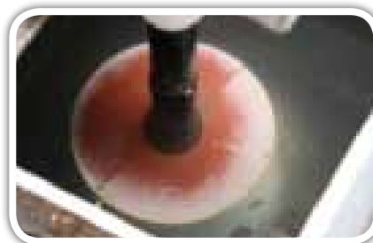
Picture 2 Disc with reddish-brown antifouling
